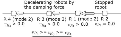
Fig. 4. Interaction Force Exerted against All the Robots behind Stopped Robot
