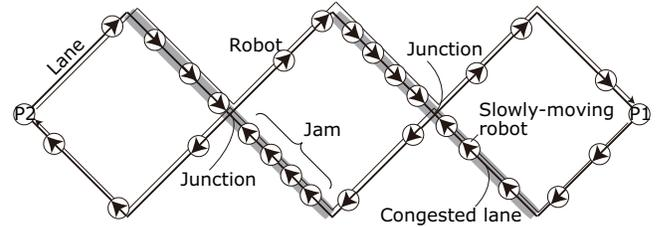
Fig. 6. Schematic Example of Jams of Robots Due to Bottlenecks
