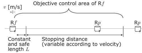
Fig. 1. Forward Objective Area for Position-Based Bang-Bang Control
