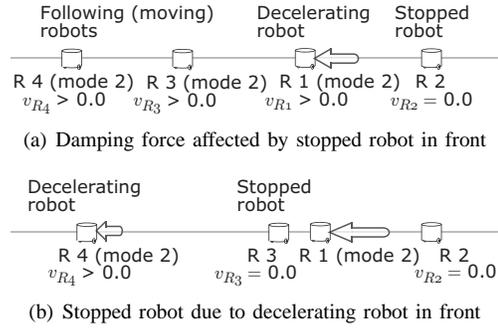
Fig. 3. Problem of Previous Robot Behavior Control Technique
