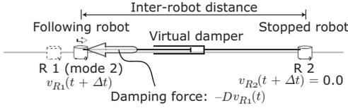
Fig. 2. Control Scenario with Virtual Damper for Interaction Force
