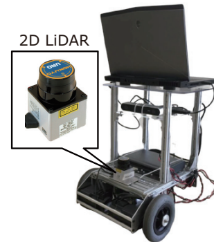
Fig. 1 Mobile robot equipped with 2D LiDAR
